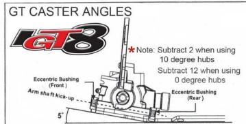
Adjust the front caster angle by changing the "Eccentric Bushing" on the front lower arm.
